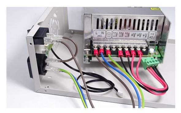
⑤ Assemble the switch power supply: Install the switch power supply on the lower board
