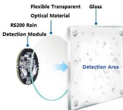
Figure 2.3 Side View of Module Installation Layers
