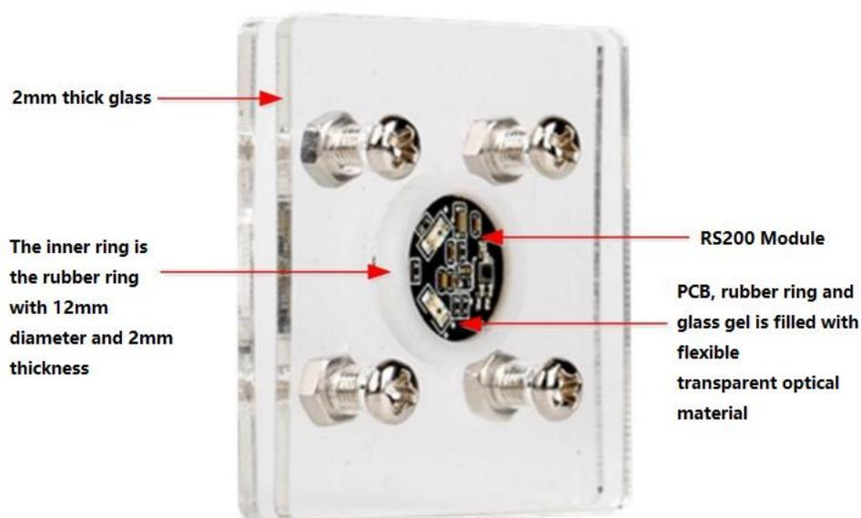
Figure 2.4 Final Installation Effect
