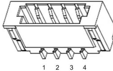
Figure 2.1 Wire-to-Board Socket
