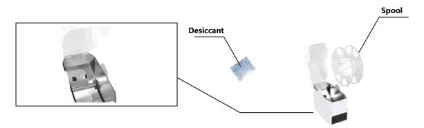
4. Put the spool in and pull the filament out through the outlet, close the cover. (The direction to pull filament can be bottom-up, or from top to bottom, depending on the position of printer)
